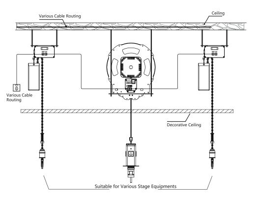
(Installation diagram; GSPC 12 is not a load-bearing product.)
