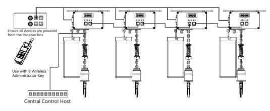
When using multiple devices together, connect a compatible receiver and use with a Wireless Administrator Key. As shown in the diagram, connect the first device to the receiver and the other end of the receiver to the Central Control Host. Connect the remaining devices to each other. Power all devices from the receiver. (Built-in wiring is for four suspension points and one wire collector.)
